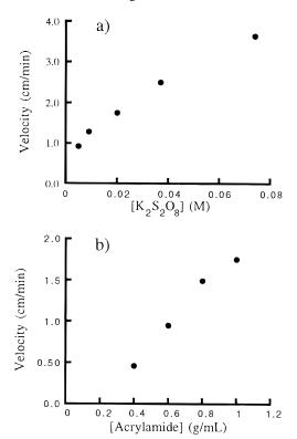
Figure 2. (a) The velocity dependence on initiator concentration with a fixed 20 g of acrylamide in 20 mL of DMSO solution. (b) The velocity dependence on acrylamide concentration (g/mL of DMSO) with a fixed persulfate concentration of 0.018 M (0.020 g/20 mL).
